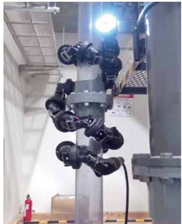
Pipe Climbing of Snake Robot
