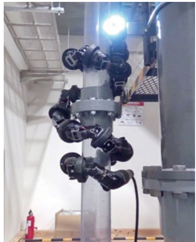
Pipe Climbing of Snake Robot
