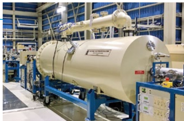
An electrostatic accelerator for MeV-energy ion beams (Radiation Laboratory in Uji campus)
