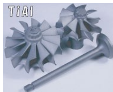
High temperature structural Materials: Turbo charger rotors and an engine valve of TiAl-based alloy
