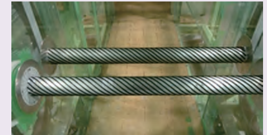
Wind-tunnel test using a model of parallel cables with spiral protuberances
