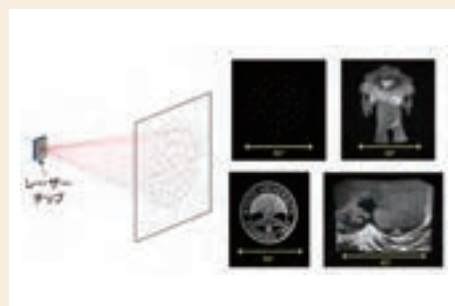
Schematic diagram of a PCSEL capable of directly emitting various beam patterns, and examples of emission patterns. We successfully generated beam patterns including multi-dot patterns, the mascot for EXPO 2025 Osaka, the Kyoto University logo, and one of the Thirty-Six Views of Mt. Fuji.
