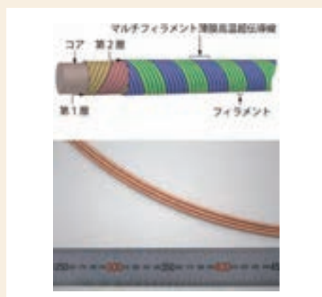
SCSC cable (Top: conceptual diagram; bottom: enlarged view of an actually fabricated 5 m long SCSC cable)
