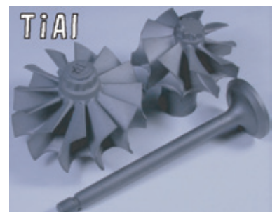
High temperature structural Materials: Turbo charger rotors and an engine valve of TiAl-based alloy
