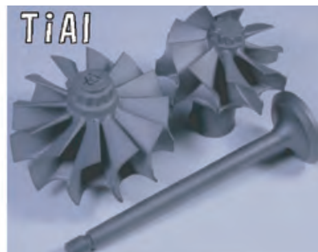
High temperature structural materials - Turbo charger rotor of TiAl-based alloy
