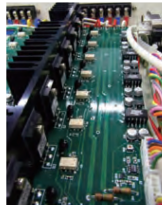
Power integrated circuits (power router) based on SiC
