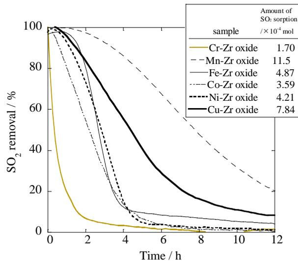
**Figure 1.** SO<sub>2</sub> removal by *M*-Zr oxide (*M* = Cr, Mn, Fe, Co, Ni, Cu, *M/Zr* = 1). Reaction conditions: 1000 ppm SO<sub>2</sub>, 10% O<sub>2</sub>, He balance; *T* = 200°C; *W/F* = 1.0 g s cm<sup>-3</sup>. The samples were calcined at 450°C in air.
